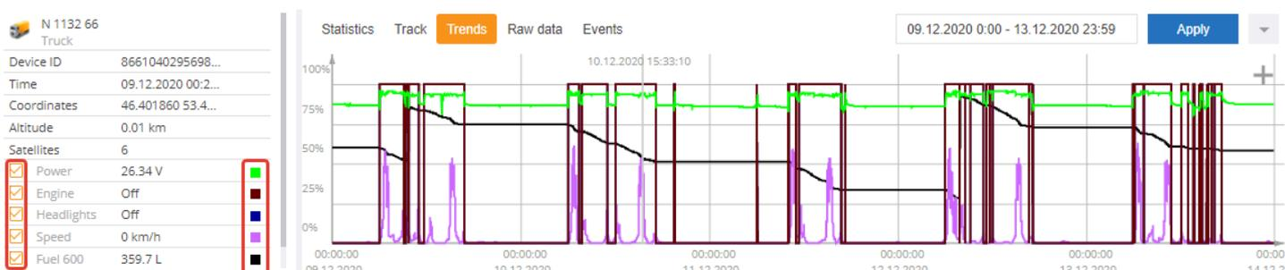
Check the checkboxes in the panel on the left to enable/disable the display of the parameters (fuel data, ignition on/off, engine power, etc.) for a particular object. The colored box opposite a certain parameter corresponds to the color of the curve on the graph.
